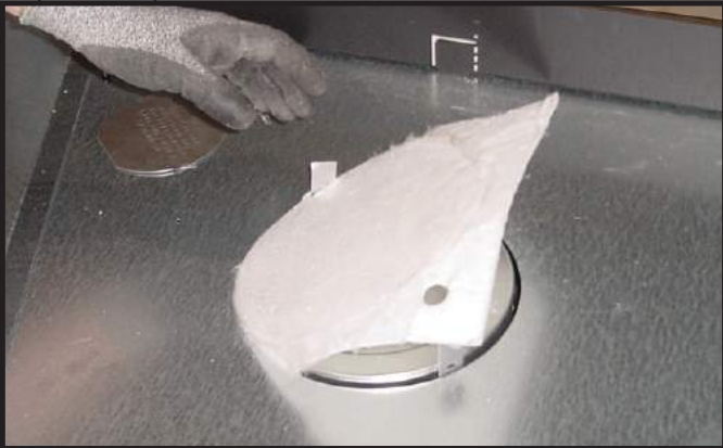
Figure 6.2 (Generic Appliance Shown) Remove the white gasket material covering the seal cap.
