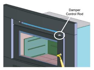
Install the draft plate cover by sliding the tabs into the tab brackets on the inside top of the firebox, ensure the damper control rod fits through the opening in the draft plate cover.
