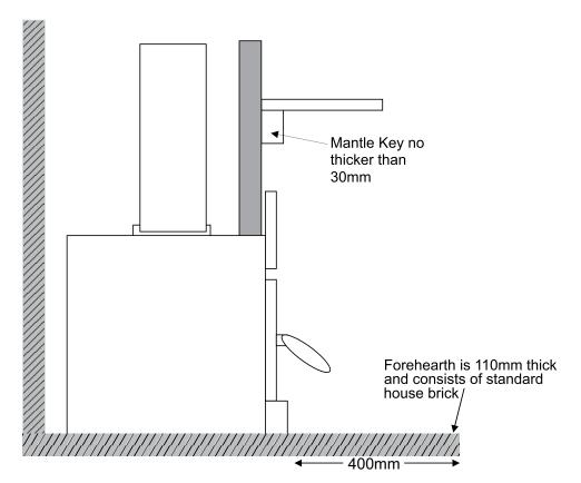
NOTE - If using 30mm cement sheet the hearth will need to extend to 820mm
