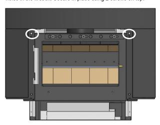
4. Install the fan fascia by aligning the bottom screw locations with the bottom faceplate. See page 13 for fan wiring diagram.
