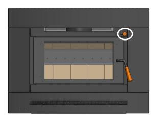
7. Install knob on damper control rod.
