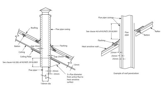
Example of sloped ceiling penetration Figure 10
