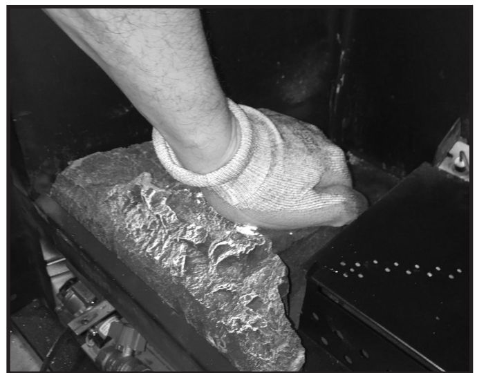
Figure 11.2 Press Left Hearth Firmly Into Place
