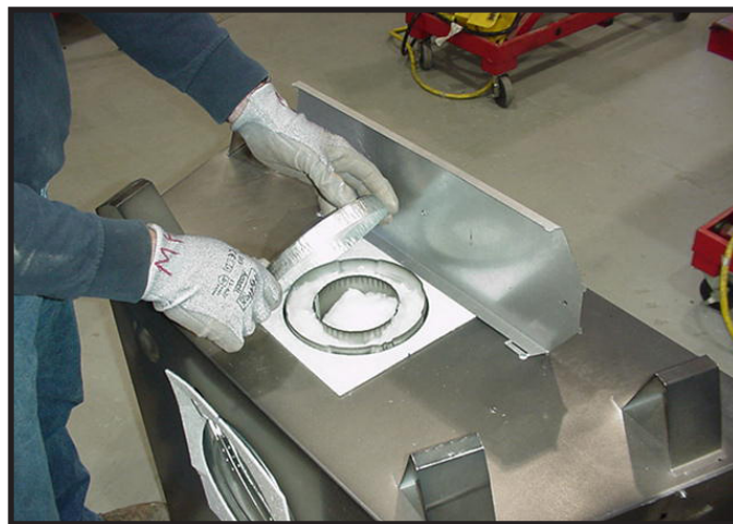
Figure 6.4 Remove the seal cap.
