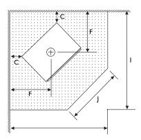
NOTE: The Hearth is not required to sit flush against the rear wall.
