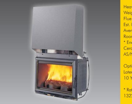
Heavy duty cast iron wood heater Weight : 185 kgs Flue size : ø 200 mm Est. Heat Output power : 25 Kwh Average smoke temperature : 314 °C Room size : 50 - 100 m2 \* Energy efficiency rating : 74.5% Ceramic glass 820°C heat resistant AS/NZS 4013 Tested
