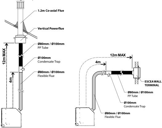
**Vertically Terminated:** (utilises the escea vertical power flue enclosure kit)
