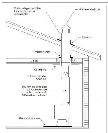
If the draft is insufficient or periodic down drafting occurs and the heater smokes or only burns slowly, extending the flue or fitting a specialist cowl will usually resolve the issue.
