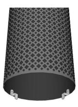
Place the first length of 150mm active flue into the flue spigot of the heater. With the 900mm inner shield fitted inside the decro-mesh with the spacers attached, slide the decro-mesh over the active flue. Locate the tabs of the "Z" spacers between the flue spigot and the active flue.
