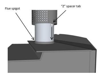
Warning: Do not install the locating ring if supplied with the decro-mesh kit as this will restrict the air flow. If the draft is insufficient or periodic down drafting occurs and the heater smokes or only burns slowly, extending the flue or fitting a specialist cowl will usually resolve the issue.
