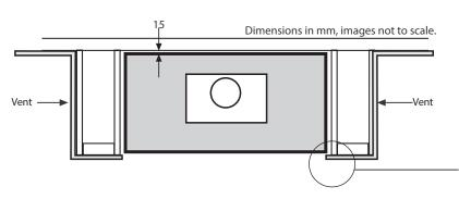
Villaboard can overlap clearance gap between ZCB and frameing, and run the over front of ZCB. Do not silicon or adhere villaboard to ZCB as heat expansion of ZCB will cause cracking.
