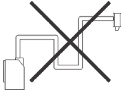
U style flue runs must not be installed
