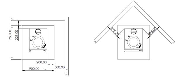
Figure 5 Bakeheart Minimum Clearance to Combustibles
