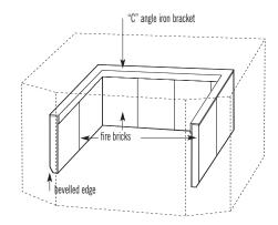
Now place one extra firebrick on either side of the firebox to complete the installation of the firebricks. (i.e. two each side and remainder on the back wall.)
