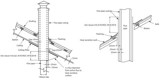
Figure 7 REFERENCE: AS2918:2018 FIGURE 4.6 - TYPICAL EXAMPLE OF A SLOPED PENETRATION FOR AN UNTESTED FLUE-SYSTEM
