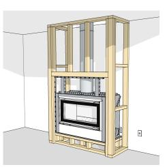
Install the fireplace on the base or structure following the TC950 Installation Manual. Restrain the fire to its base. Fit the top panel and standoffs for the Zero Clearance Kit. Install the Skamotec fixing brackets to the perimeter of the cavity opening.
