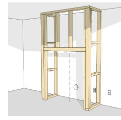
A location is selected with electrical supply adjacent. Allow for an isolation switch outside the cavity. Obtain flue centreline to ensure the flue run is clear from
