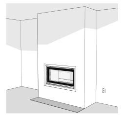
Complete the installation by installing the remaining fireplace components, apply any finishes to the walls, and install the floor protector or hearth.
