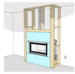
Install the flue and liners to the correct configuration and height.
