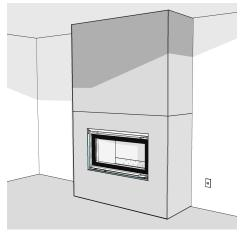
Fix the fibre cement sheet substrate to the framework.
