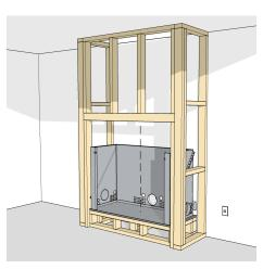
Install the structural base for the fireplace **40mm** behind the face of the timber framing.
