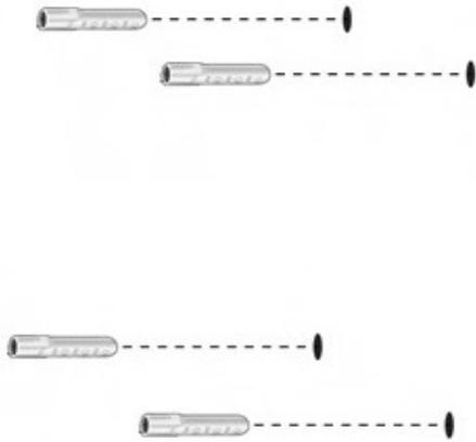
Mark and drill four holes for the wall mounting bracket in the wall and insert the corresponding dowels into the holes. (Dowels are not provided)
