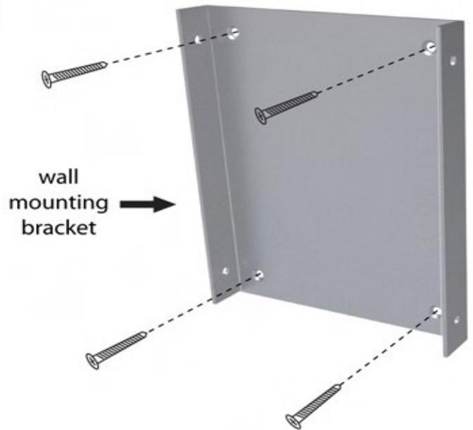
Fix the wall mounting bracket on the wall with screws. (Screws are not provided)
