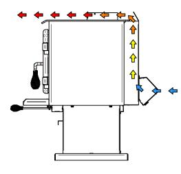
Figure 7: Air flow with a blower
