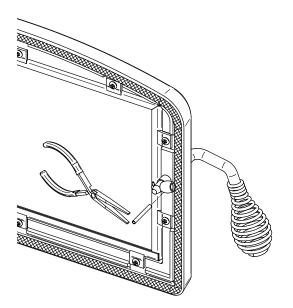
Figure 10: Removing the split pin
