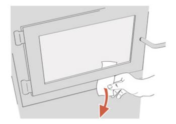
Figure 9: Door gasket seal verification
