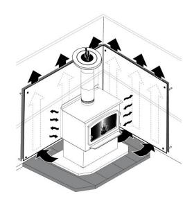
Figure 13: Heat shield
