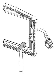
Figure 11: Installing the split pin
